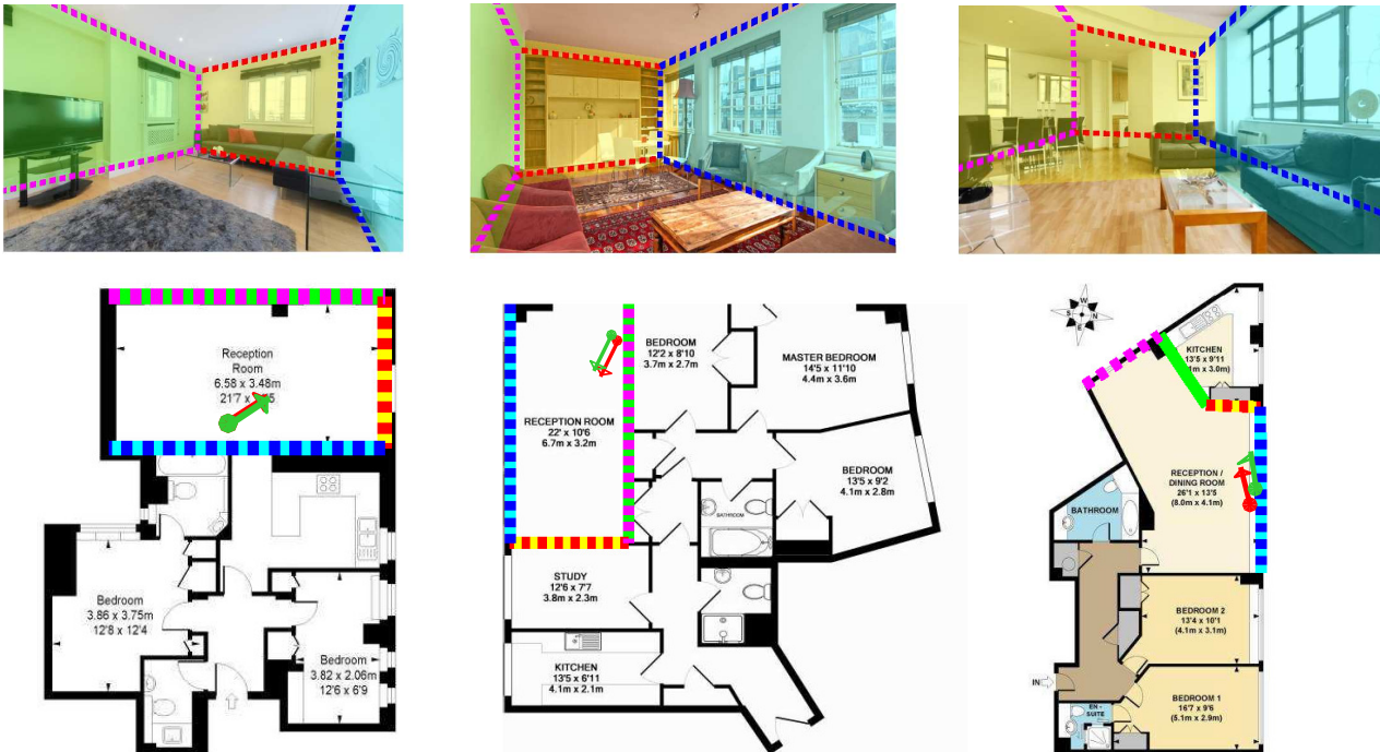
Figure 9. Room layout estimation and room-apartment alignment with our model. The top row of images color code the estimated vertical walls, and ground-truth layout is shown with dashed lines. In the bottom row, we show the floor plans with predicted and GT alignments. The solid colors show the alignment predicted by the model, where the yellow solid line denotes the alignment prediction for the front face. Similarly, GT alignment is shown with dashed lines. A red point shows the GT location of the camera, and the arrow is the viewing direction. Green point and line is our estimated localization. On the right we show a failed example due to a weird shape of the room.
